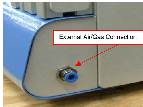
Figure 2: External Air/Gas supply on the back of TF 2500
